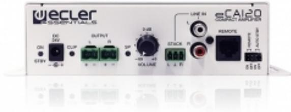
Ecler ESSENTIALS eCA120 is a 2 x 60 WRMS @ 4 Ω stereo micro-amplifier, in a very compact format and a light and silent (fanless) design. It features 1 LINE ST input (RCA/Euroblock), AUTO STANDBY function and volume remote control, compatible with Ecler WpMVOL and WpMVOL-SR wall panels (0-10 VDC). Auto-standby function. External, universal and CE/UL/CCC certified power supply. Dimensions: 190 x 48 x 90mm. Weight 600 g.
